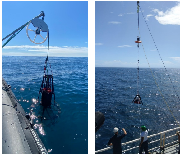
Fig. 3: Left: TNO experimental dipping sonar, right: NILUS node. From [2].
